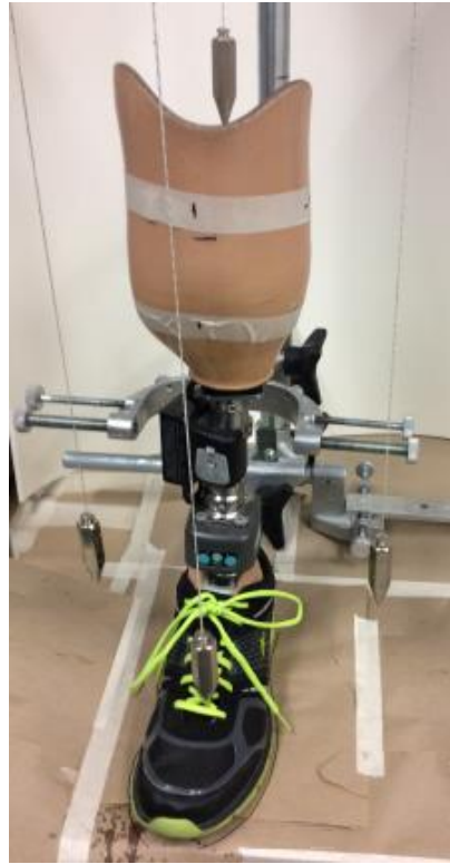
Figure 2: preserving the original alignment with parallel plumb lines
