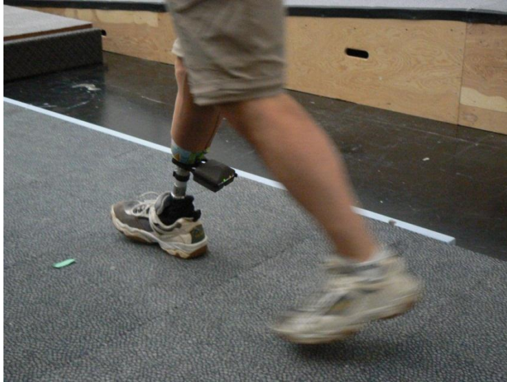
Figure 10 Collection of force and moment data with clear view of Europa ™
