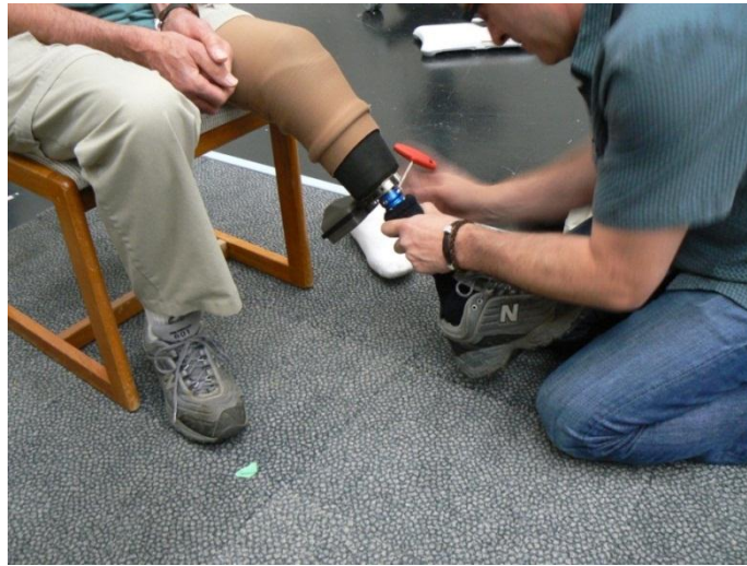
Figure 8 Attachment of a study foot to Smart Pyramid™ and socket with Europa™ data logger visible
