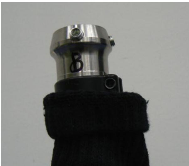
Figure 3 Sock was tied off just below the adaptor with a zip tie.
